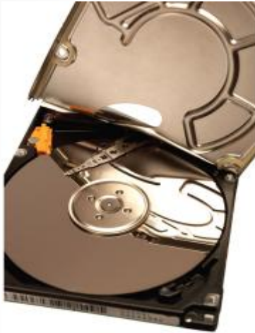
Hard drive with enclosure opened
